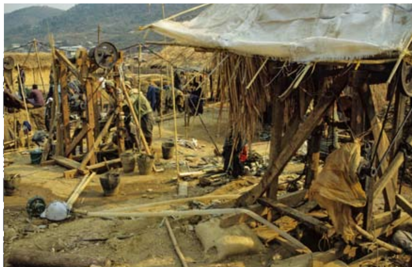
Fig. 5. Two of the lebin shafts at Kyatpyin. Each is 30 m deep, and ventilation is provided by air pumped through the plastic piping that emerges from the carrier-bag 'junction box'.
