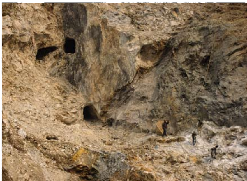
Fig. 12. Old tunnel mines are exposed in the marble at the Linyaungchi mine, where all the byon cover has been worked out, and the miners are now blasting into bedrock.
