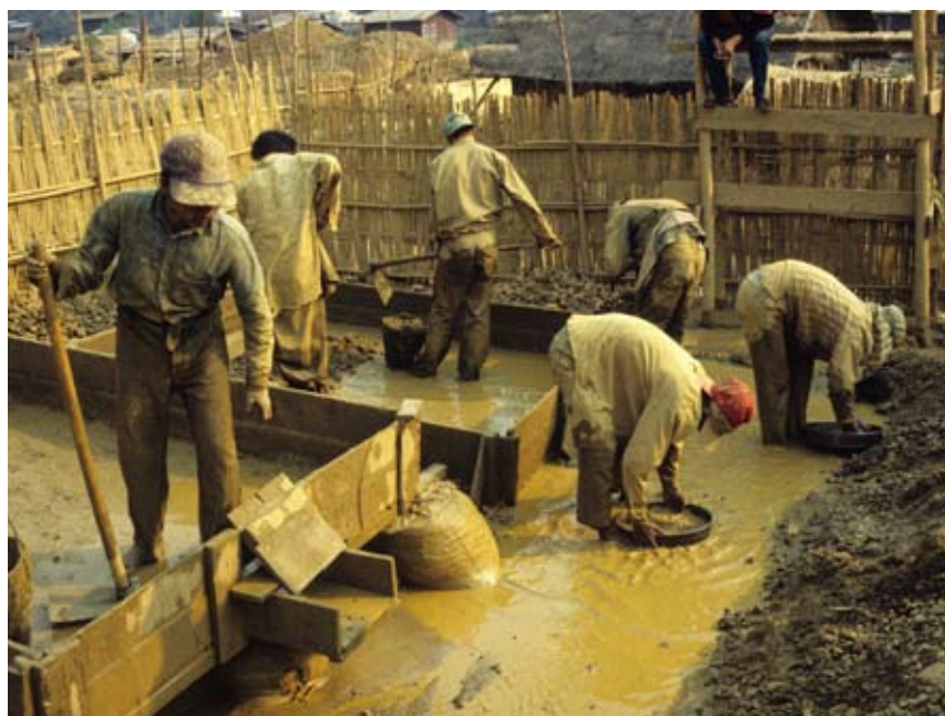
Fig. 6. Sorting the mined earth from a group of shaft mines at Kyatpyin. Rubies are concentrated at the bottoms of the sieves that are hand-shaken in water.
