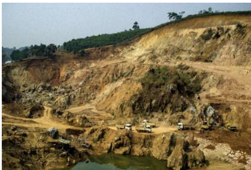
Fig. 7. The Shwepyiyae open pit. Ruby-bearing alluvial byon is excavated on the right by machines, until rockhead is reached. Byon between the rockhead pinnacles is hand worked on the left. The upper bench exposes the cover of barren red earth.
